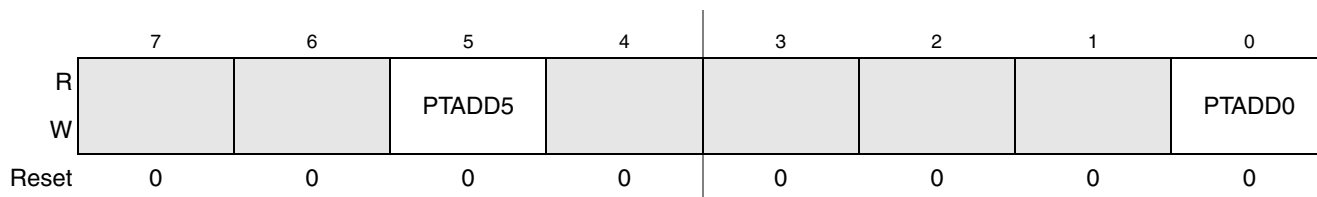
Figure 6-3. Data Direction for Port A Register (PTADD)
