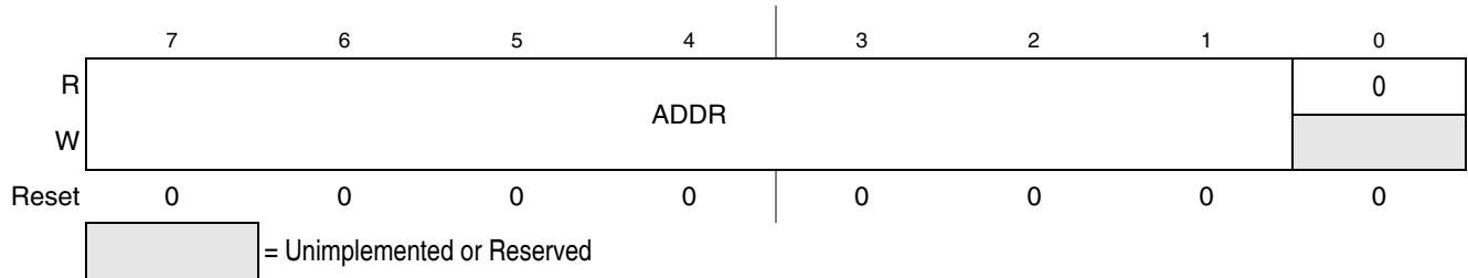
Figure 13-3. IIC Address Register (IIC1A)
