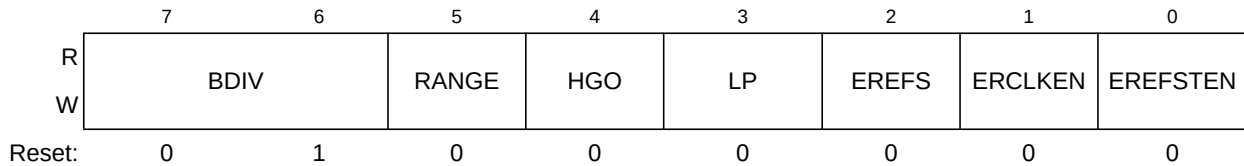
Figure 8-4. MCG Control Register 2 (MCGC2)
