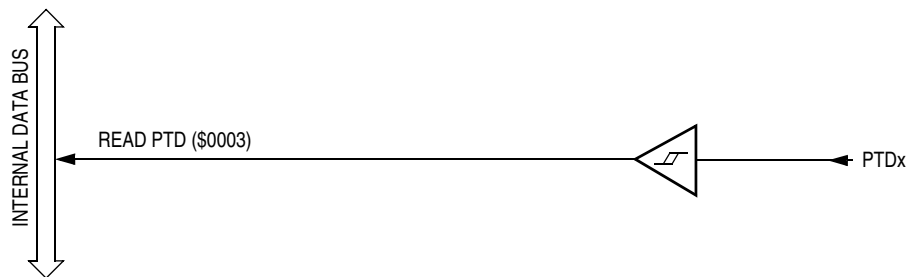
Figure 10-12. Port D Input Circuit
