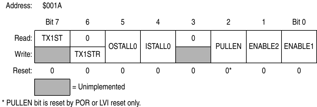
Figure 9-22. USB Control Register 3 (UCR3)
