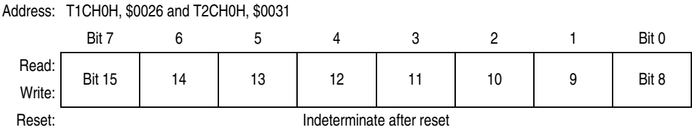
Figure 19-13. TIM Channel 0 Register High (TCH0H)
