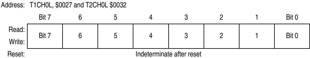
Figure 19-14. TIM Channel 0 Register Low (TCH0L)
