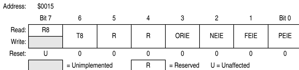
Figure 13-12. ESCI Control Register 3 (SCC3)
