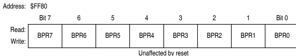
Figure 2-4. FLASH-1 Block Protect Register (FL1BPR)
