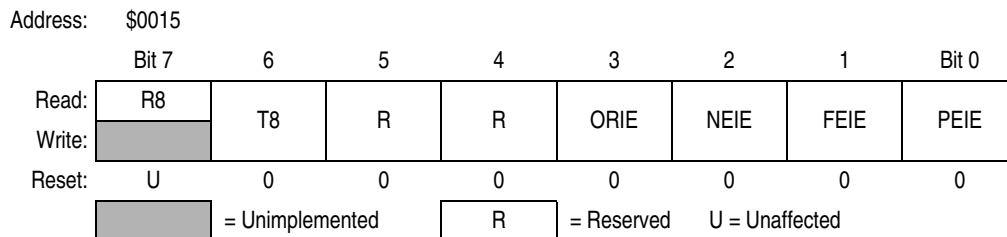
Figure 14-12. ESCI Control Register 3 (SCC3)
