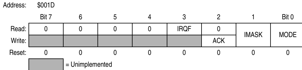
Figure 8-3. IRQ Status and Control Register (INTSCR)
