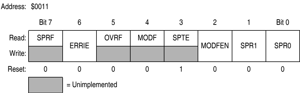
Figure 16-14. SPI Status and Control Register (SPSCR)
