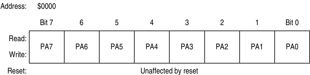
Figure 6-2. Port A Data Register (PORTA)
