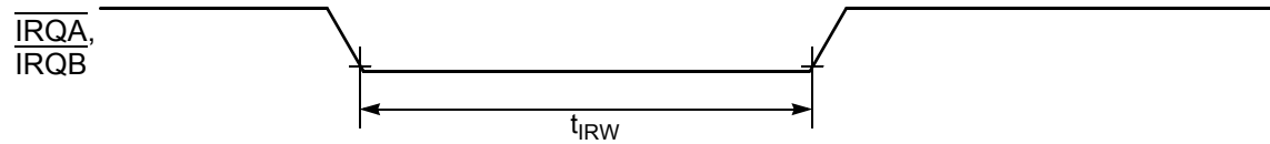
Figure 10-6 External Interrupt Timing (Negative Edge-Sensitive)
