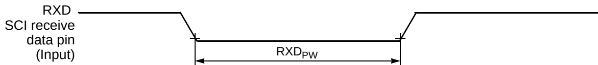
Figure 10-15 RXD Pulse Width
