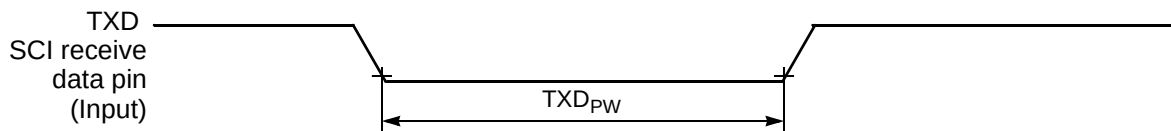
Figure 10-16 TXD Pulse Width
