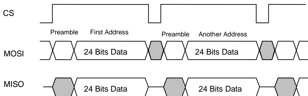
Figure 3. SPI Transfer Protocol Multiple Read/Write Access
