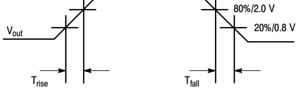
Figure 14. Waveforms: Rise and Fall Times
