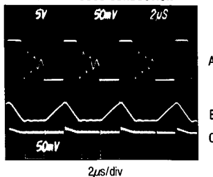
SWITCHING WAVEFORMS DISCONTINUOUS CONDUCTION
