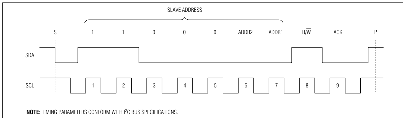
Figure 1. MAX3544 Slave Address Byte. Example shows read address 0x0C1 (ADDR pin grounded).
