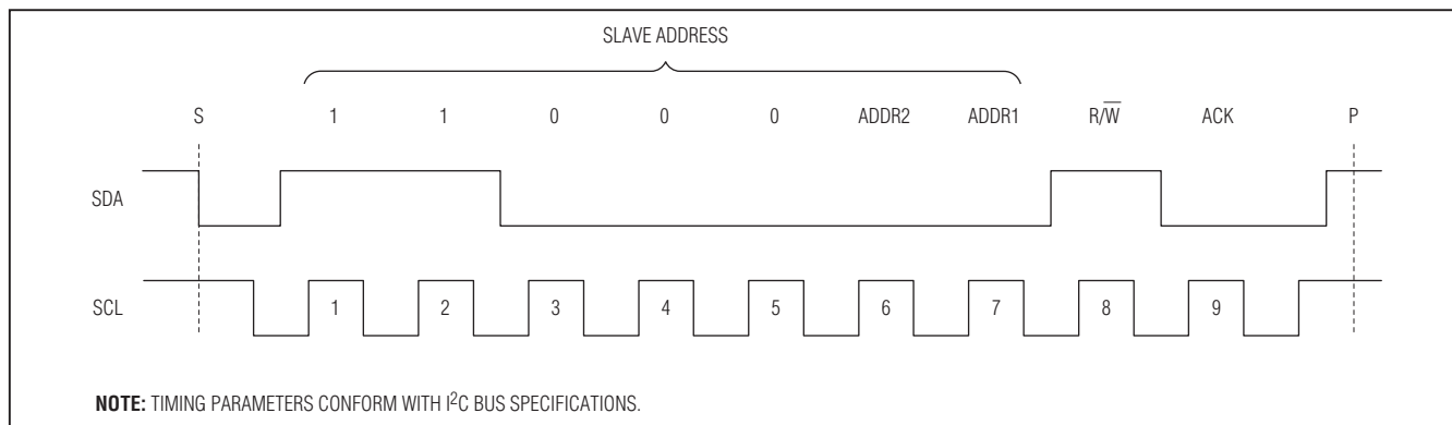
Figure 1. MAX3543 Slave Address Byte. Example shows read address 0x0C1 (ADDR pin grounded).
