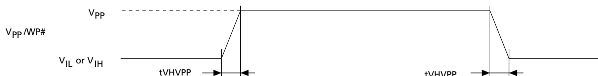
Figure 24: Accelerated Programming Timing Waveform
