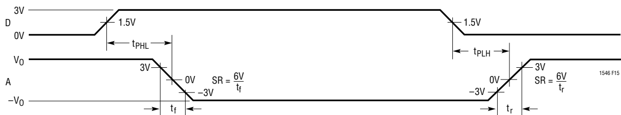
Figure 15. V.28 Driver Propagation Delays
