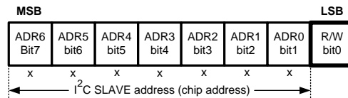
Figure 16. I 2 C Chip Address (0x2C)
