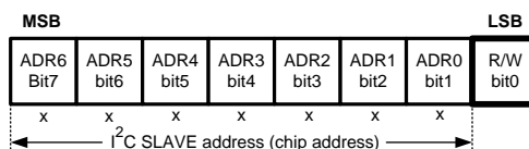
Figure 23. I 2 C Chip Address
