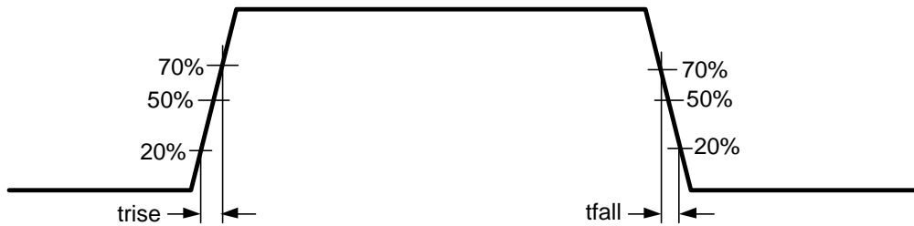
Figure 4. Output Transition Time (A and B Side)
