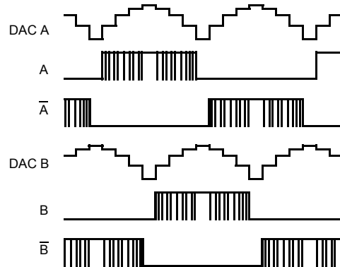
Figure 11: Stepper Motor Waveform - LM9833 Signals
