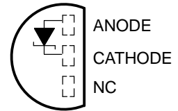
1.2 V . . . LP (TO-92/TO-226) PACKAGE (TOP VIEW)
