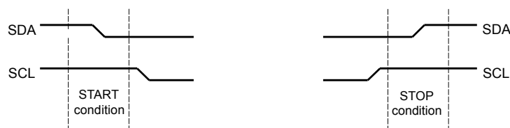
Figure 15-3. START and STOP Conditions
