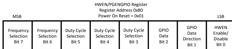
Figure 45. HPG Register Description
