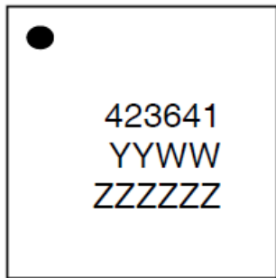
Figure 14. PE423641 package marking specification
