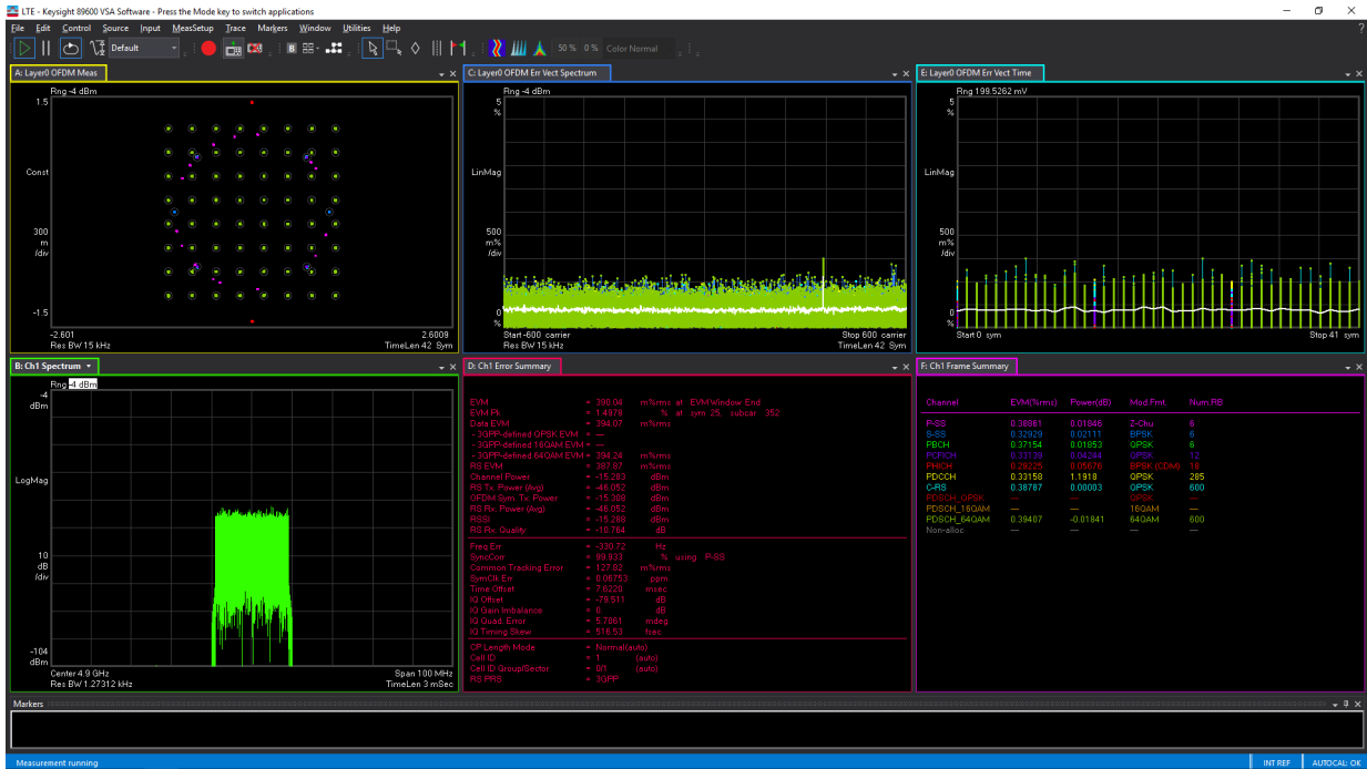
Figure 5-521. TX 20-MHz LTE Error Vector Magnitude at 4.9 GHz
