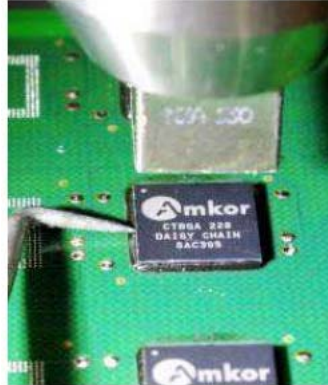
Figure 10-7: Removing Underfill Using Steel Probe
