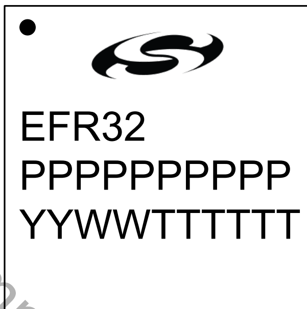
Figure 8.3. QFN32 Package Marking
