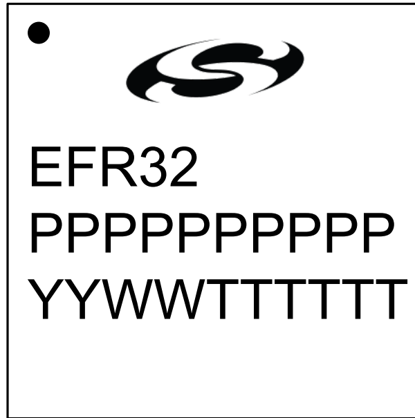
Figure 8.3. RQFN32 Package Marking
