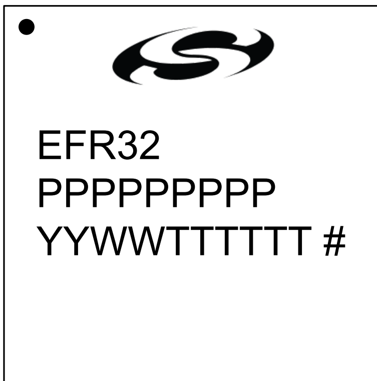
Figure 7.3. QFN48 Package Marking
