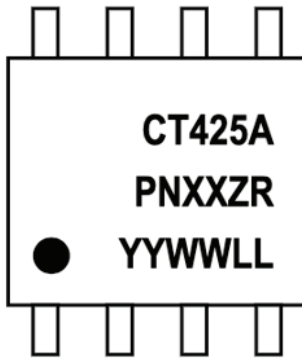
Figure 22: CT425 Device Marking for 8-lead Package
