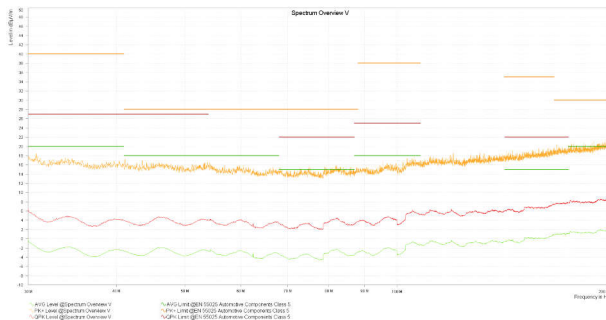
Figure 8-28. Conducted EMI versus CISPR25 Limits (Purple: Peak Signal, Green: Average Signal), LMR60440QEV
