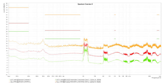
Figure 8-27. Conducted EMI versus CISPR25 Limits (Purple: Peak Signal, Green: Average Signal), LMR60440QEV
