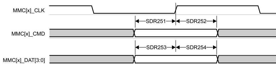
Figure 7-97. MMCSD1 – UHS-I SDR25 – Receive Mode
