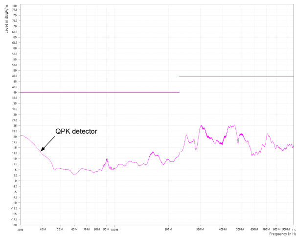
Figure 9-10. CISPR 32 Class B Radiated Emissions: Horizontal Polarization
