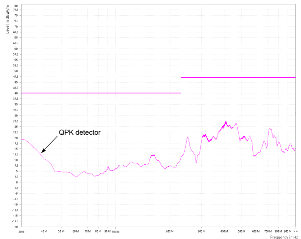
Figure 9-11. CISPR 32 Class B Radiated Emissions: Vertical Polarization
