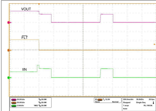
V_{IN\_SYS} = 24\text{ V} MODE connected to GND (Auto-Retry) R_{ILIM} = 9\text{ k}\Omega
