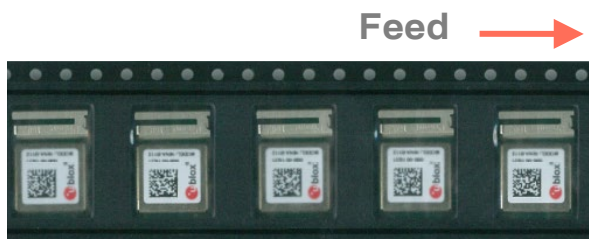
Figure 14: Orientation of NINA-W152/NINA-W156 module on tape
