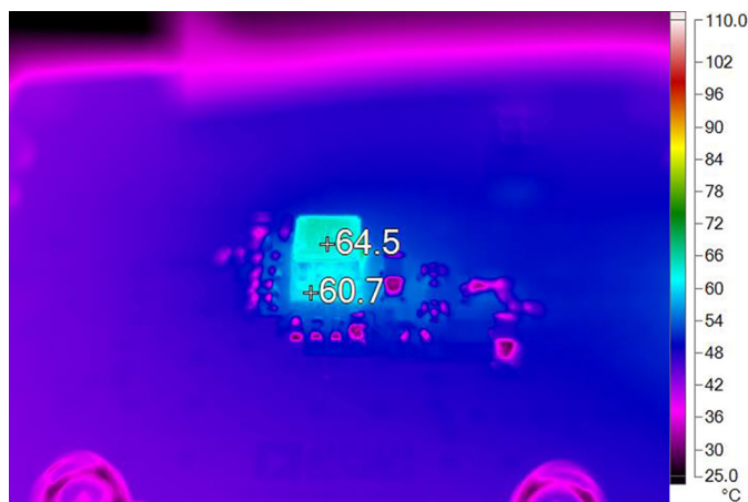
Figure 5. Thermal Image at 12V IN , 1V, 8A Output without Airflow and Heat Sink
