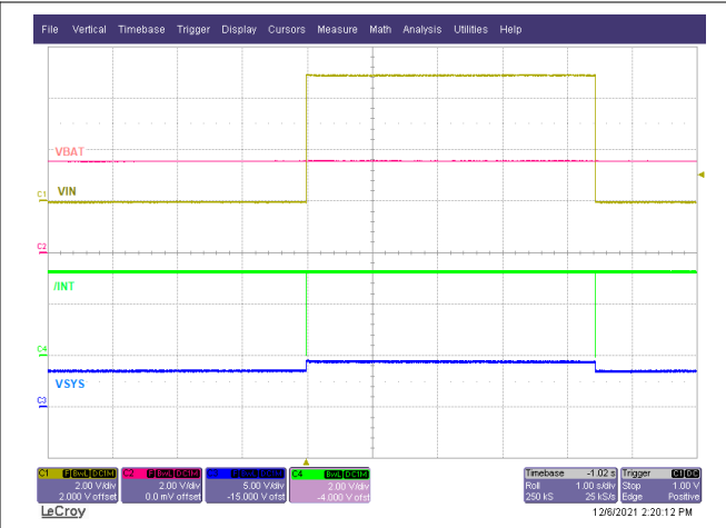
Figure 9-11. Power Good Interrupt on /INT
