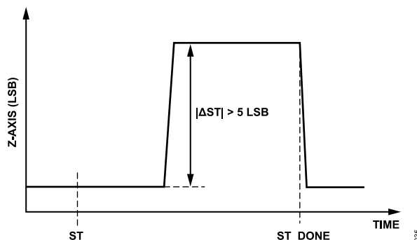
Figure 48. Self Test Waveform
