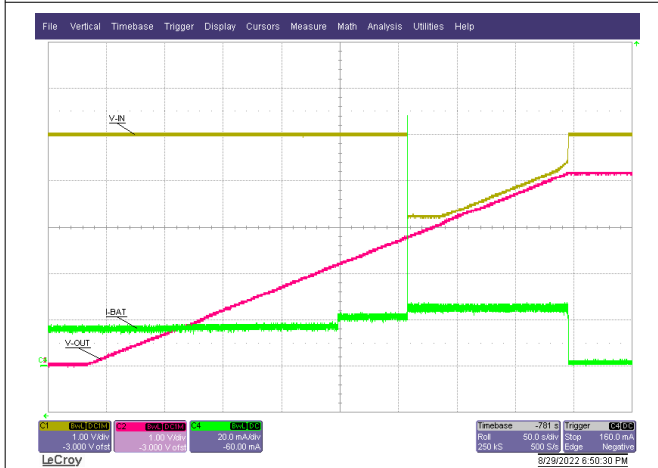
Figure 8-8. OUT Short-Circuit Response
