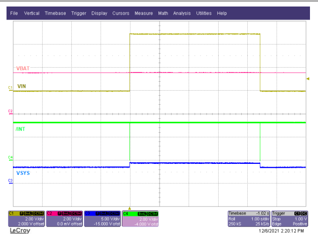
Figure 9-11. Power Good Interrupt on /INT
