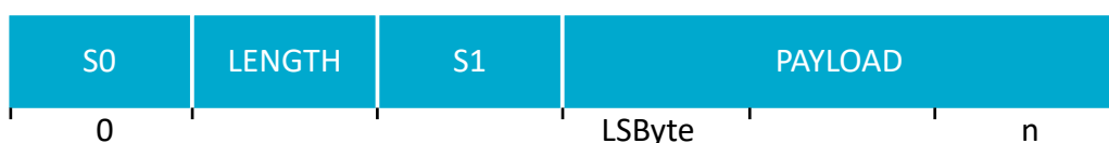
Figure 111: Representation of a RADIO packet in RAM
