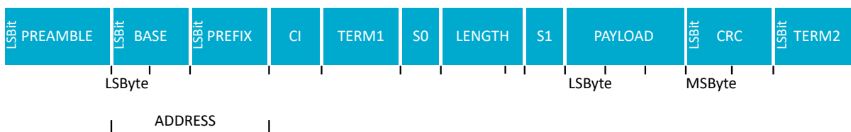
Figure 110: On-air packet layout for Long Range (125 kbps and 500 kbps) Bluetooth Low Energy modes
