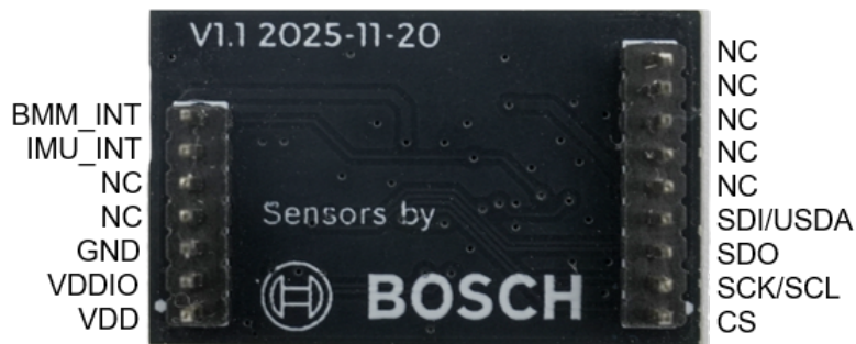
Fig. 7: ShuttleBoard-BMI270&BMM350 PCB Back View (Click to enlarge)
