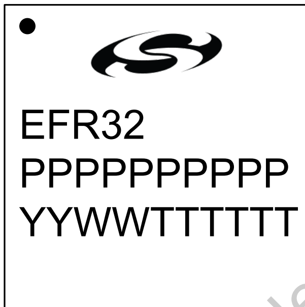
Figure 8.3. QFN32 Package Marking
