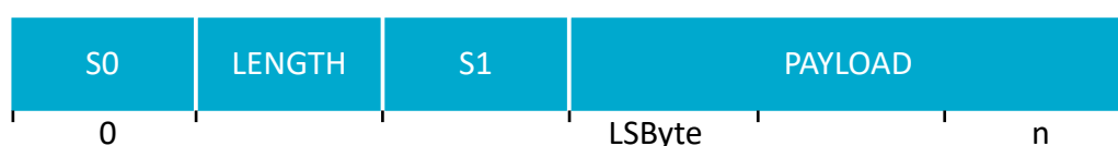
Figure 111: Representation of a RADIO packet in RAM
