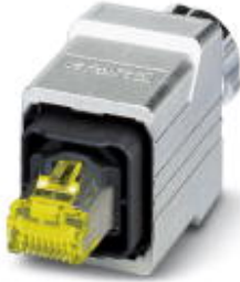
RJ45 plug-in connector, IP67, with push/pull interlocking (version 14), metal housing, for 10 Gbps, for AWG 24 ... 27 stranded conductors
