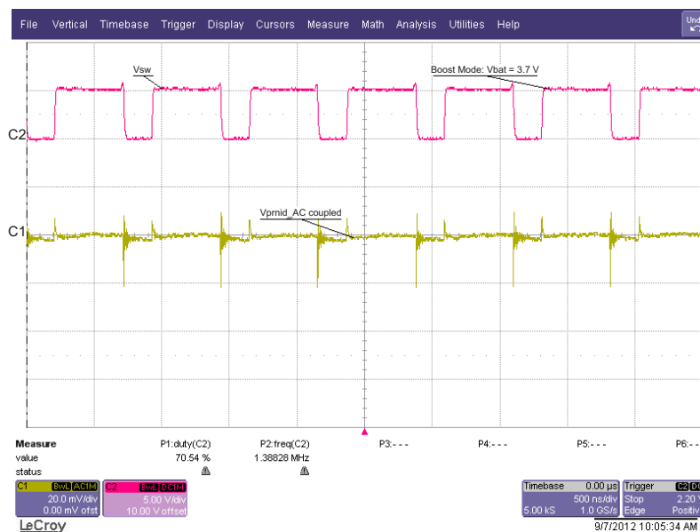
Figure 5. Boost Mode Ripple and Duty Cycle; V_{BAT} = 3.7 V
