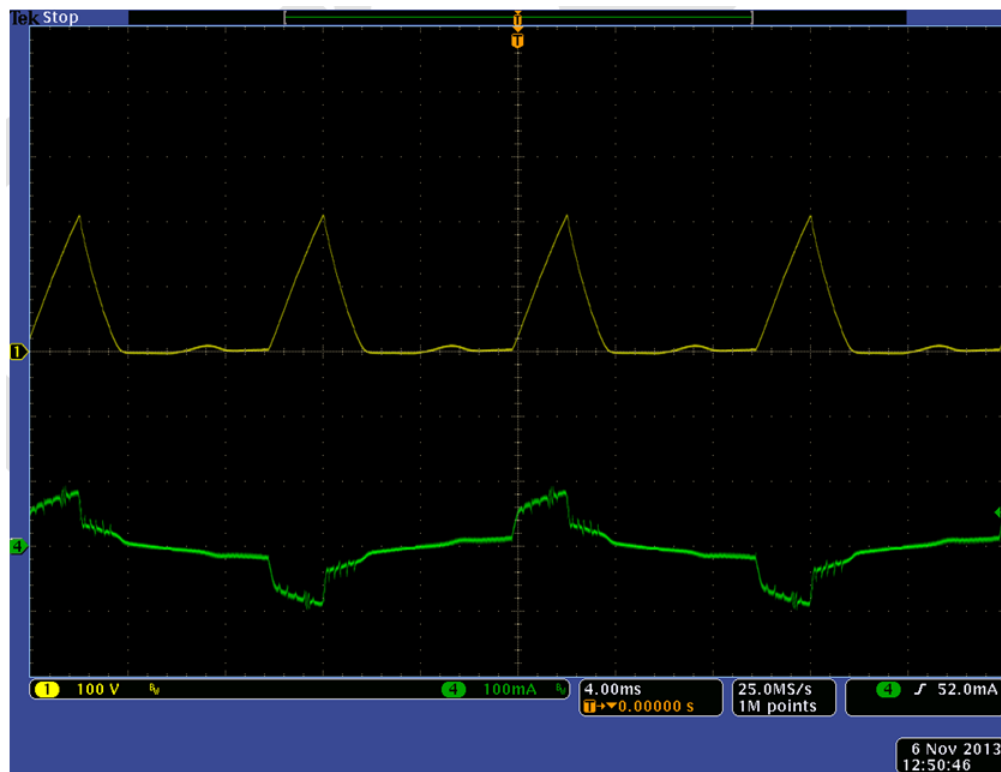
Figure 11. Reverse Phase Triac Dimming: Rectified Input Voltage (Top) and Input Current (Bottom)
